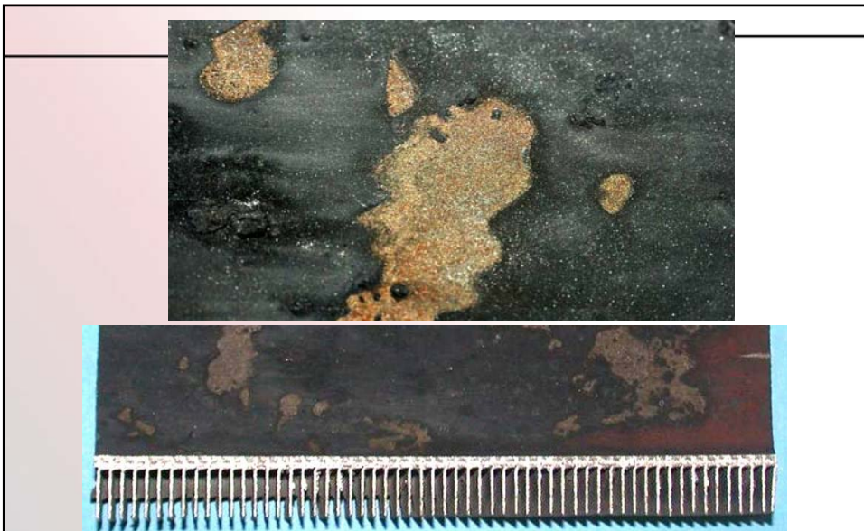
6 inch section of ACC tube and detail of the surface showing black deposits and white "bare" metal areas
