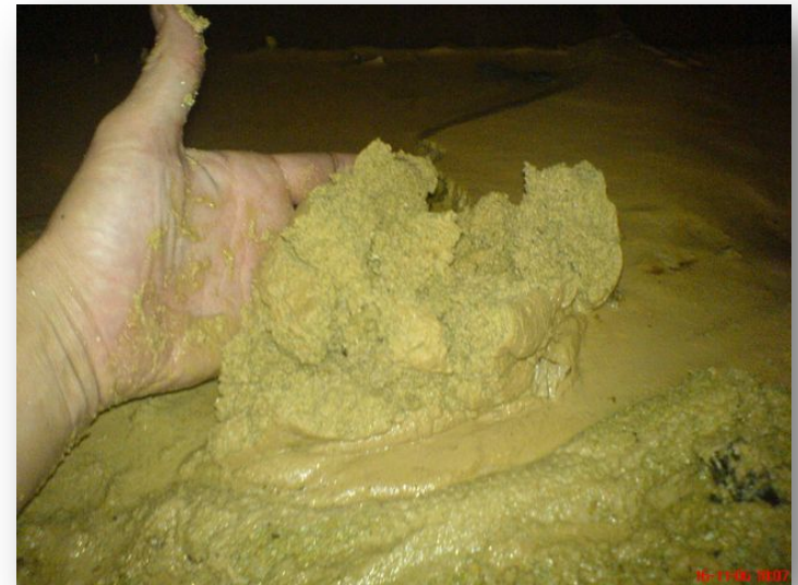
Fresh water silt removed from condenser
