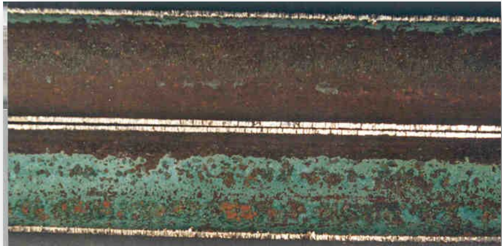
Corrosion product on copper-alloy tube
