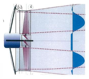
RS 725: "the pressure measurements taken show the static pressure in the chamber decreasing towards the centre of the swirling core and the average of the pressures measured in the chamber is lower than the pressure measured at the wall static tappings."
