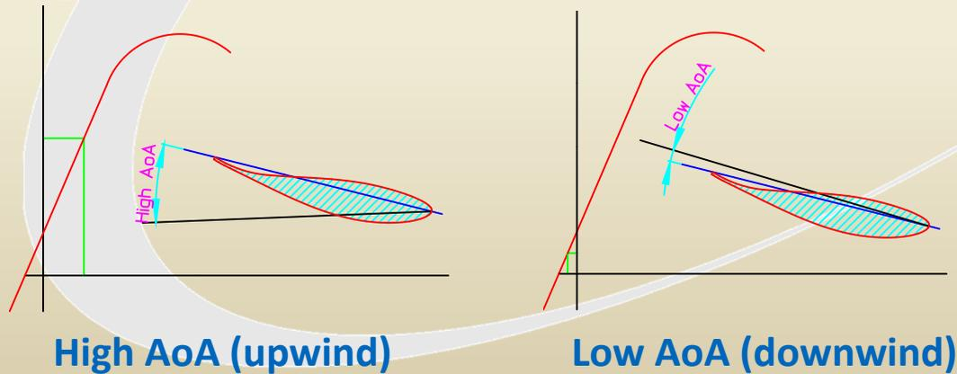
The higher the WS, the higher the AoA fluctuation with the blade position around the fan and the load variation
