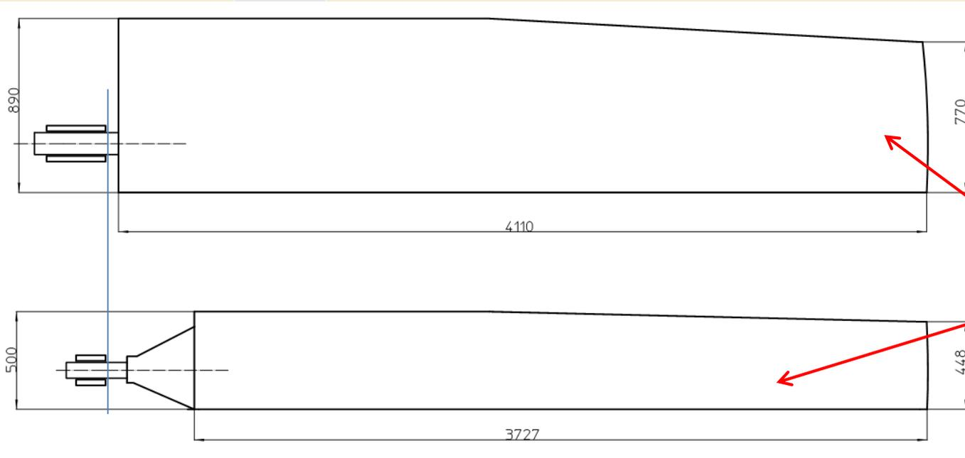
(\*) Double FRP shaft with inner friction-based damper
