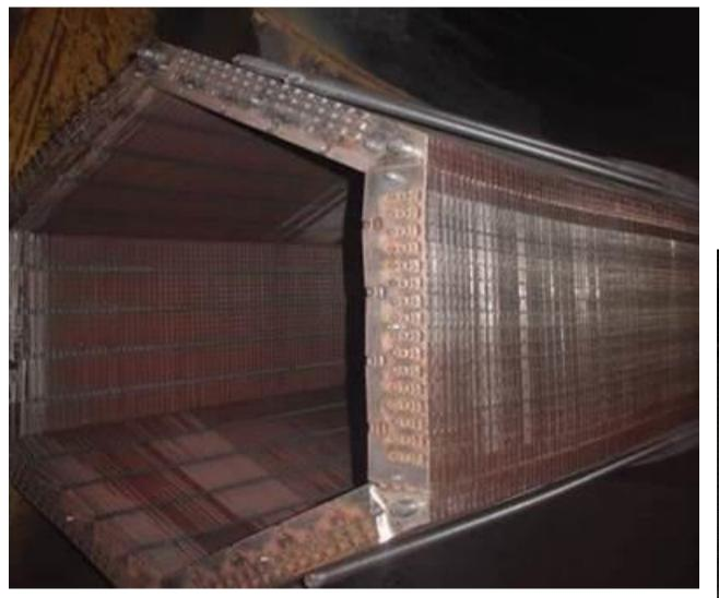
**Destroys Dump Resistor:** Elbow into duct and poor water control
