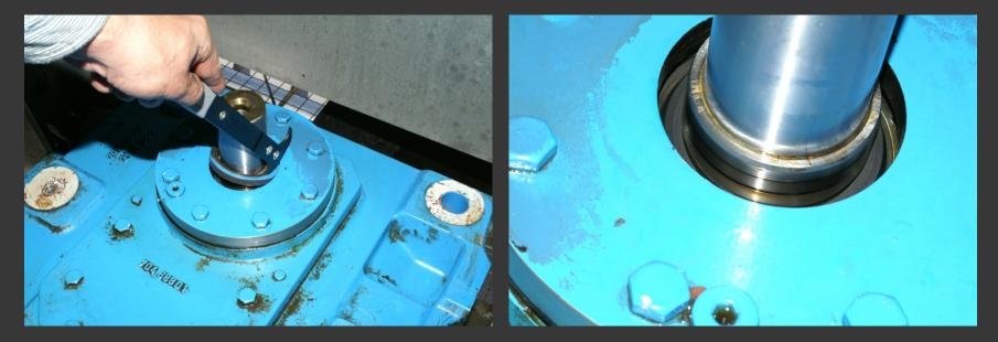
Old seal removed without removing seal plate
