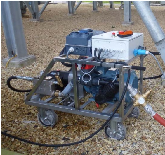
HIGH PRESSURE PUMP 22KW – 120 lpm – 130 bar
