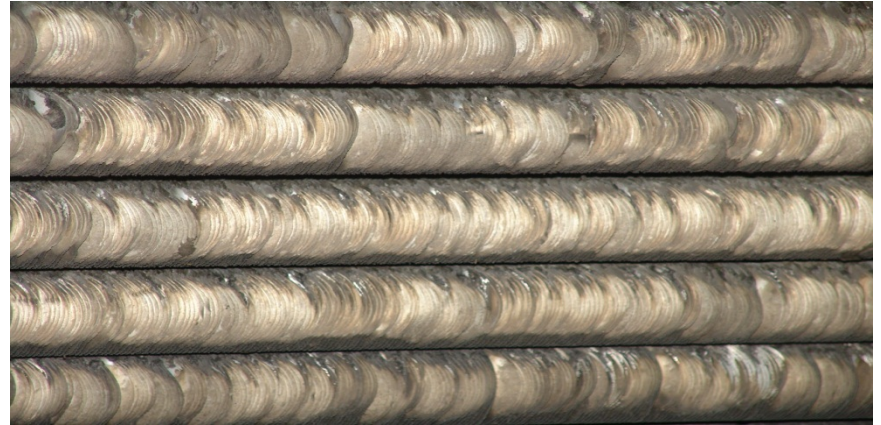
Damage by manual HP cleaning
