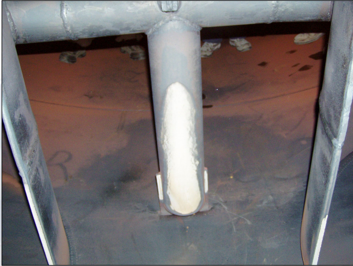
FAC on support pipe (shiny spot) at entry to lower distribution duct
