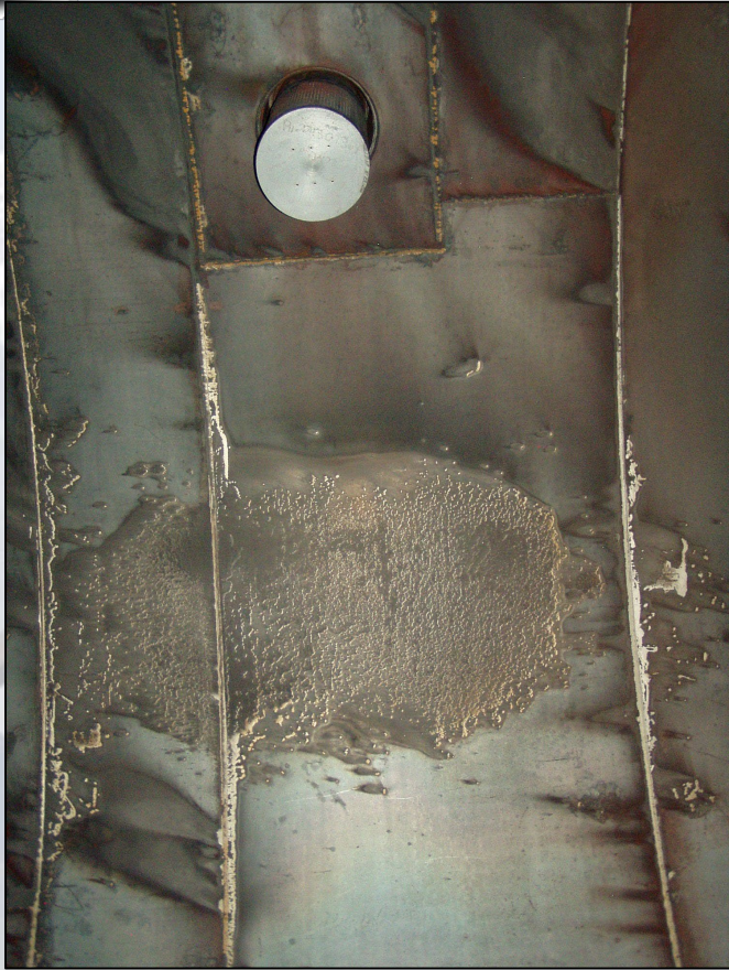
Steam bypass on top of exhaust duct, FAC at wall impact point
