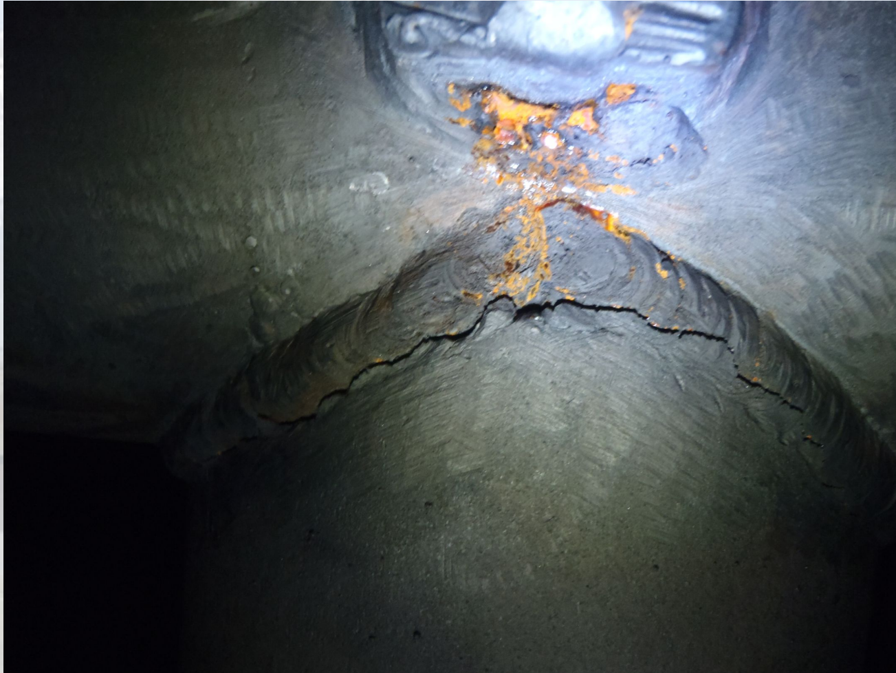
Crack at weld in turning vane support
