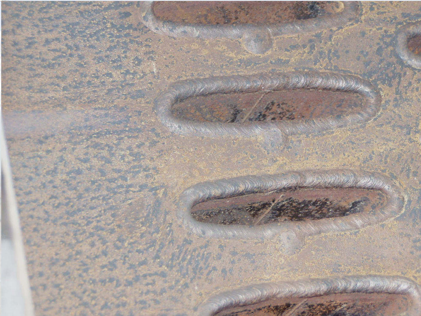
Tube inlets; area around black scale in tubes is FAC
