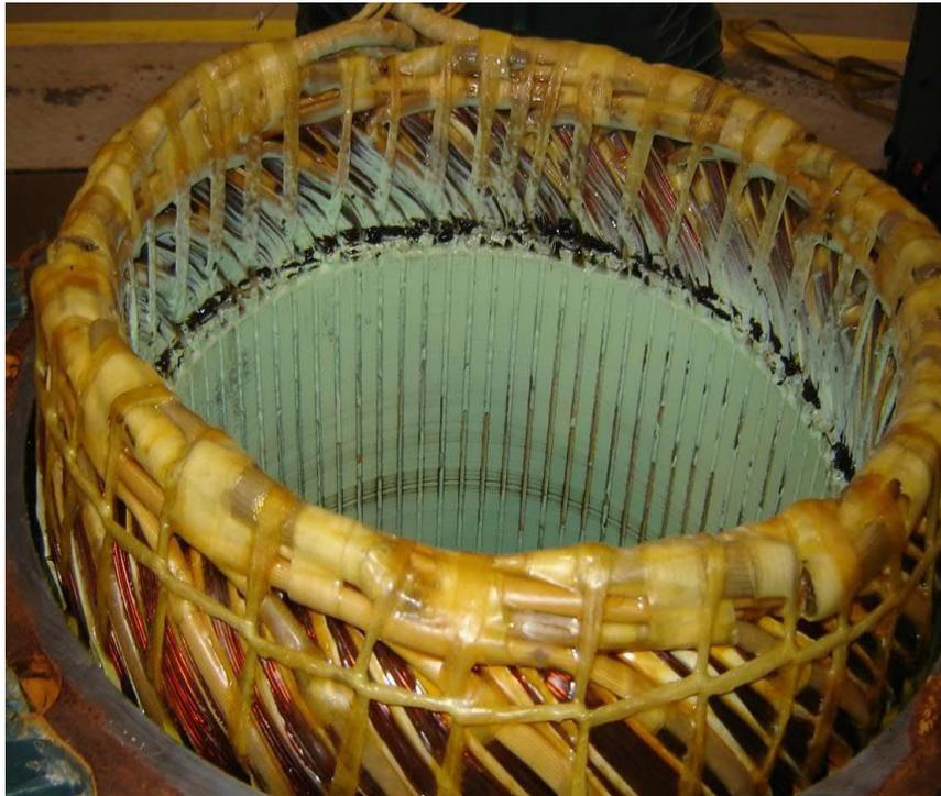
Green paint is epoxy coating for additional protection against moisture
