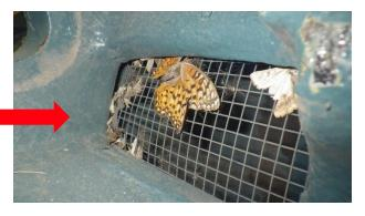
The debris is on the outside on the Exhaust Screen and appears to have been sucked in towards the motor, signaling an incorrect airflow direction.
