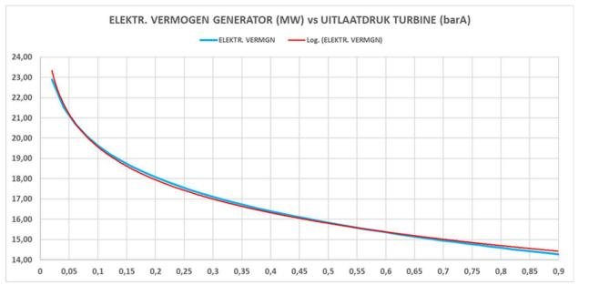
Sample from an Incinerator: Between 50 and 350 mbar, performance loss = 4.3 MW = 20.5% 0.68% per 10 mbar pressure Loss (almost 0.7%
