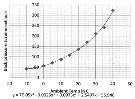
This is done for the cases 30 to 130 % duty The curves are transferred to equations to make calculations.
