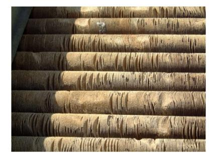
This kind of fouling either by hard water or humid dust is difficult to remove. HP water spraying will not be effective. The only way to remove this kind of fouling is blasting with calcium.
