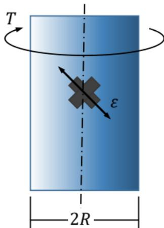
The torque strain gauges are fitted at an angle of  $45^\circ$  to the axis of the shaft. For a strain  $\varepsilon$  along the direction of the gauge the torque-strain relationship is
