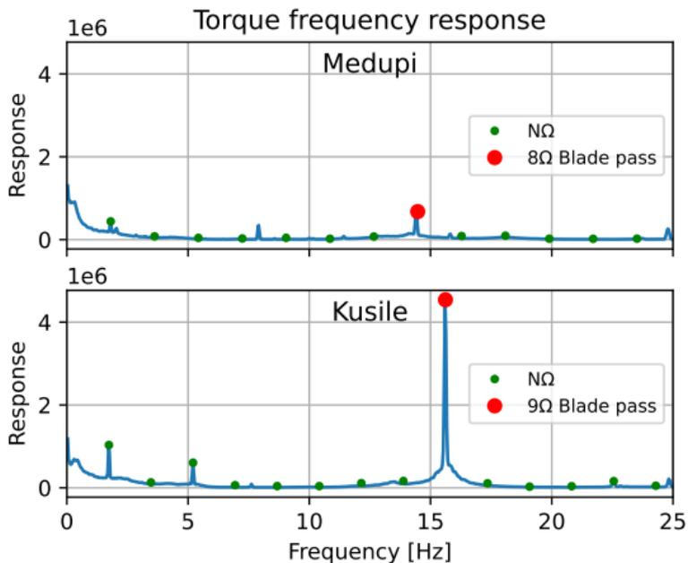
Find the average frequency response over a long time (3 hours in this instance) to smooth out noise
