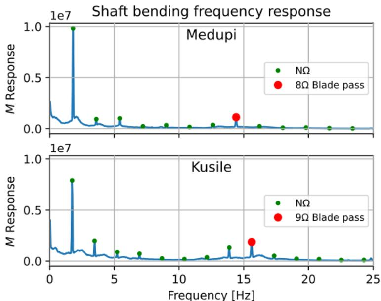
Find the average frequency response over a long time (3 hours in this instance) to smooth out noise
