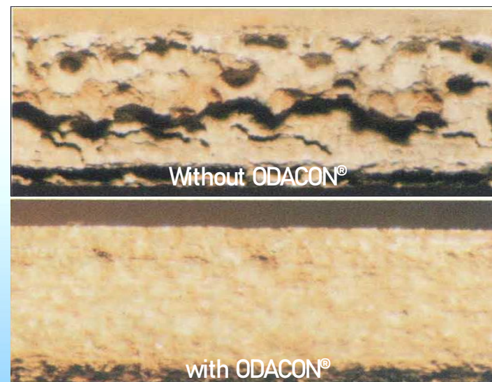
Stereo microscopic recording of samples plates in wet steam flow (magnification 1 : 12)
