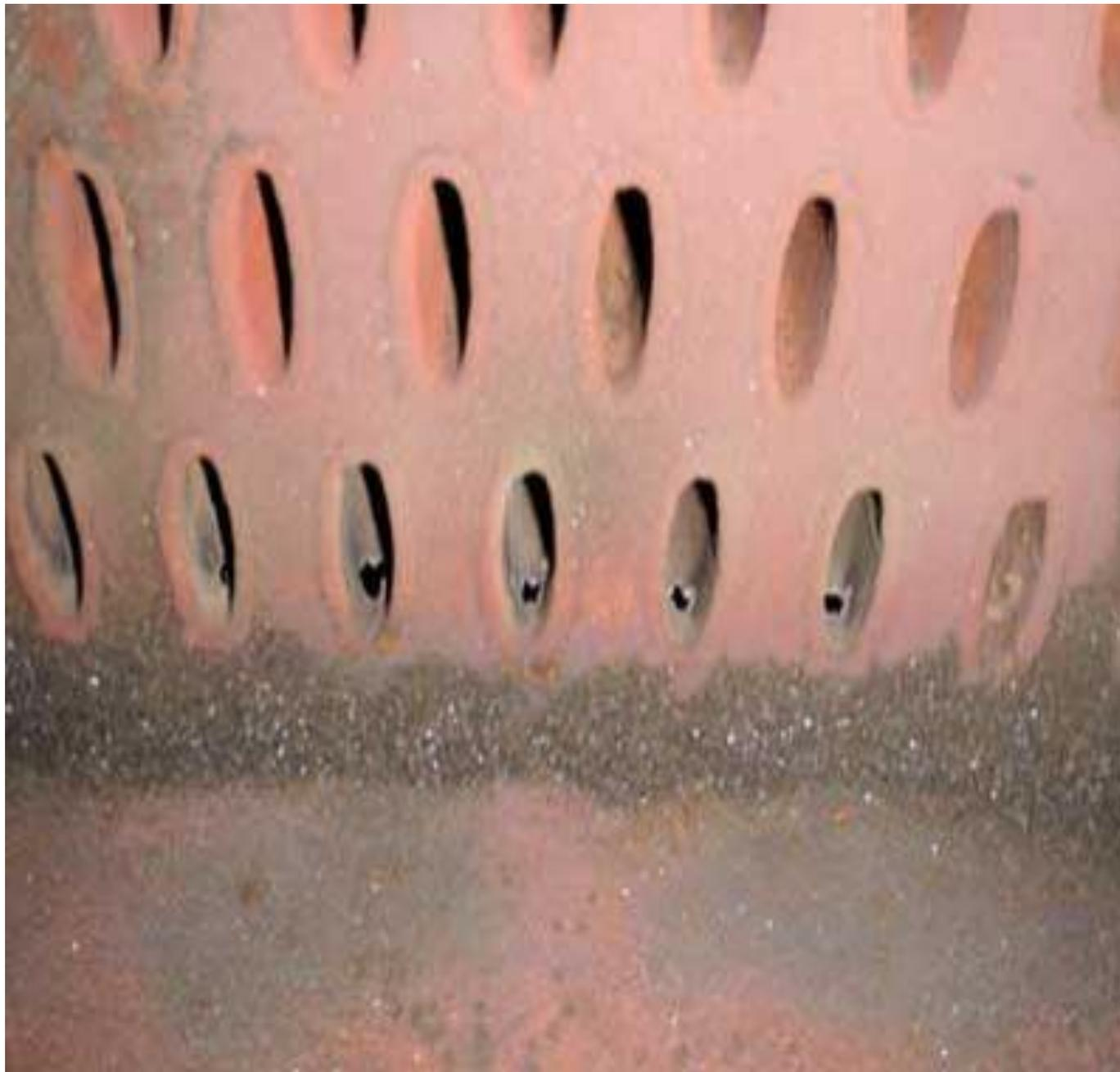
Corrosion at upper end of dephlegmators resulted in air inleakage
