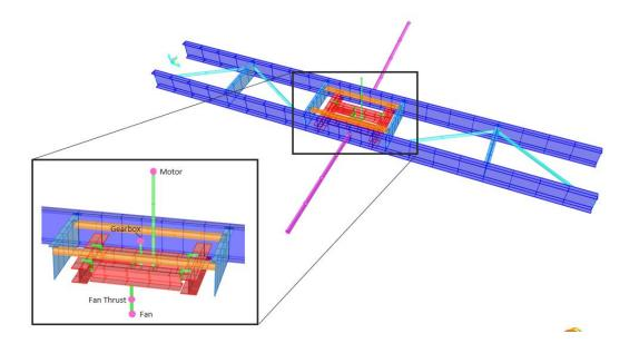
FEM Analysis confirmed primary vibration mode at 13 Hz in parallel direction on 2 speed motor modules
