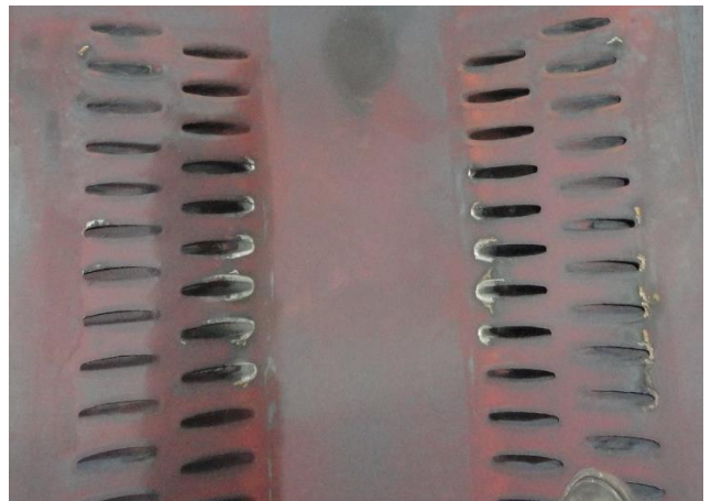
Figure 5: Finned tube entries; FAC is commonly present (bare metal areas)
