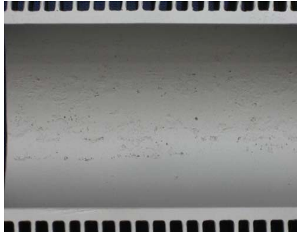
Tube after bead blast cleaning
