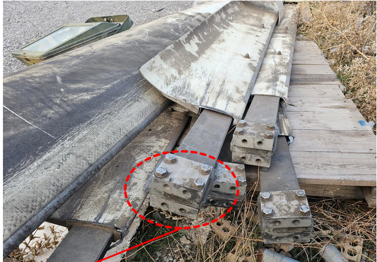
Blade shaft-to-hub connection
