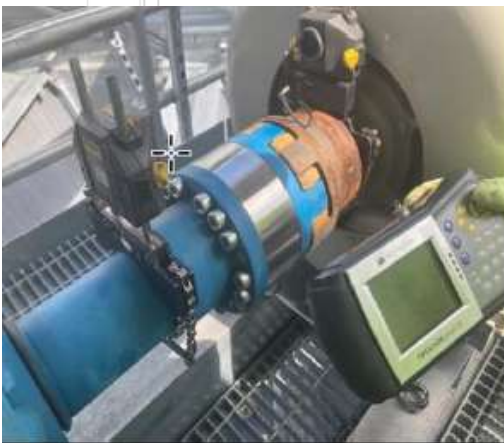
Check of alignment HSS
